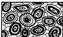
D Section of Oolitic Limestone x 20
